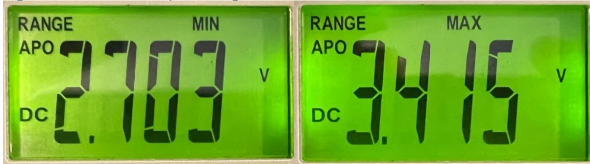
Figure 4.2.2.7 – DC Output Voltage of Ultrasonic Anemometer
