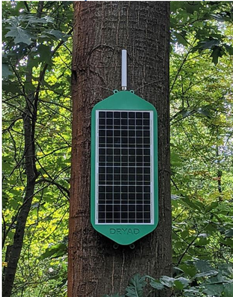
Figure 3.1.1.1 – Dryad Silvanet Mesh Gateway
