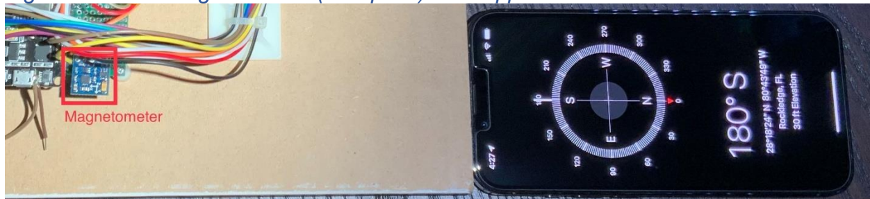
Figure 4.2.8.2 – Magnetometer (Compass) Test Apparatus
